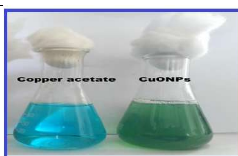
Fig. 2: Color changes before (Copper acetate) and after (CuONPs) the Cissus quadrangularis extract added.
